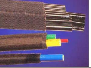
This very tough, high-quality textile sheath is particularly suitable for the hydraulic and pneumatic sectors. It can be used to bundle multiple hoses or protect a single hose. Thanks to the toughness of the material used, it has optimum resistance to mechanical stress and is compatible with oils and organic products.
